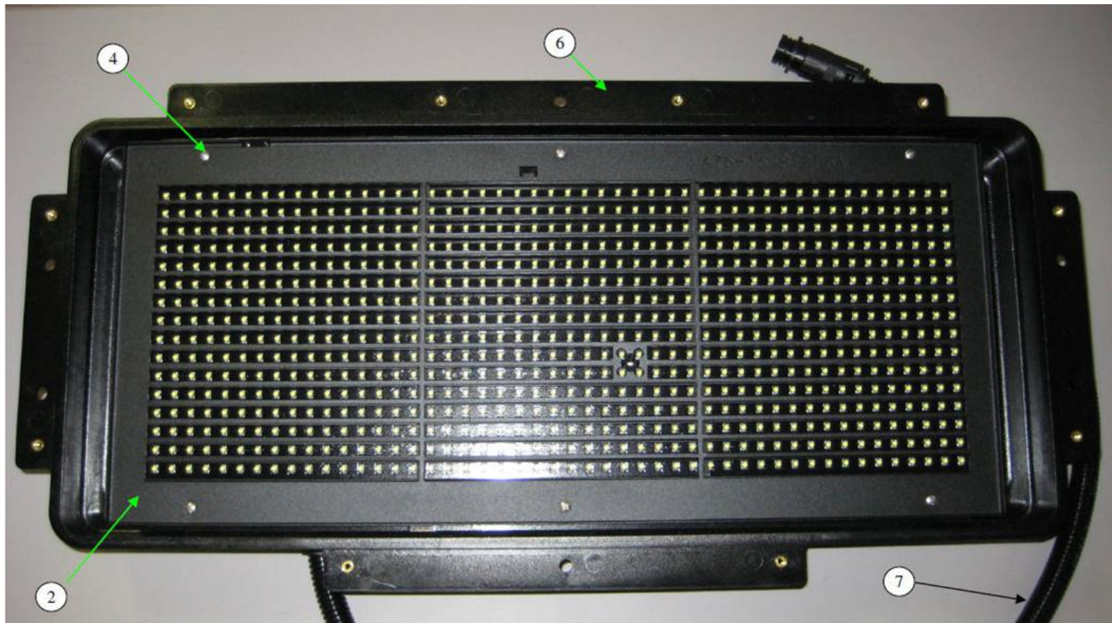
Figure 11-8. Typical Rear Sign with Cover Removed
