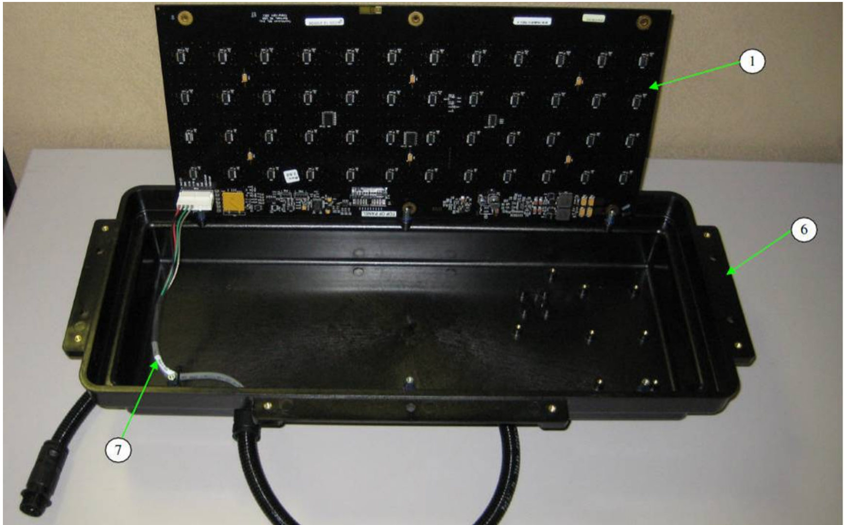
Figure 11-9. Typical Rear Sign with Cover and PWA Removed
