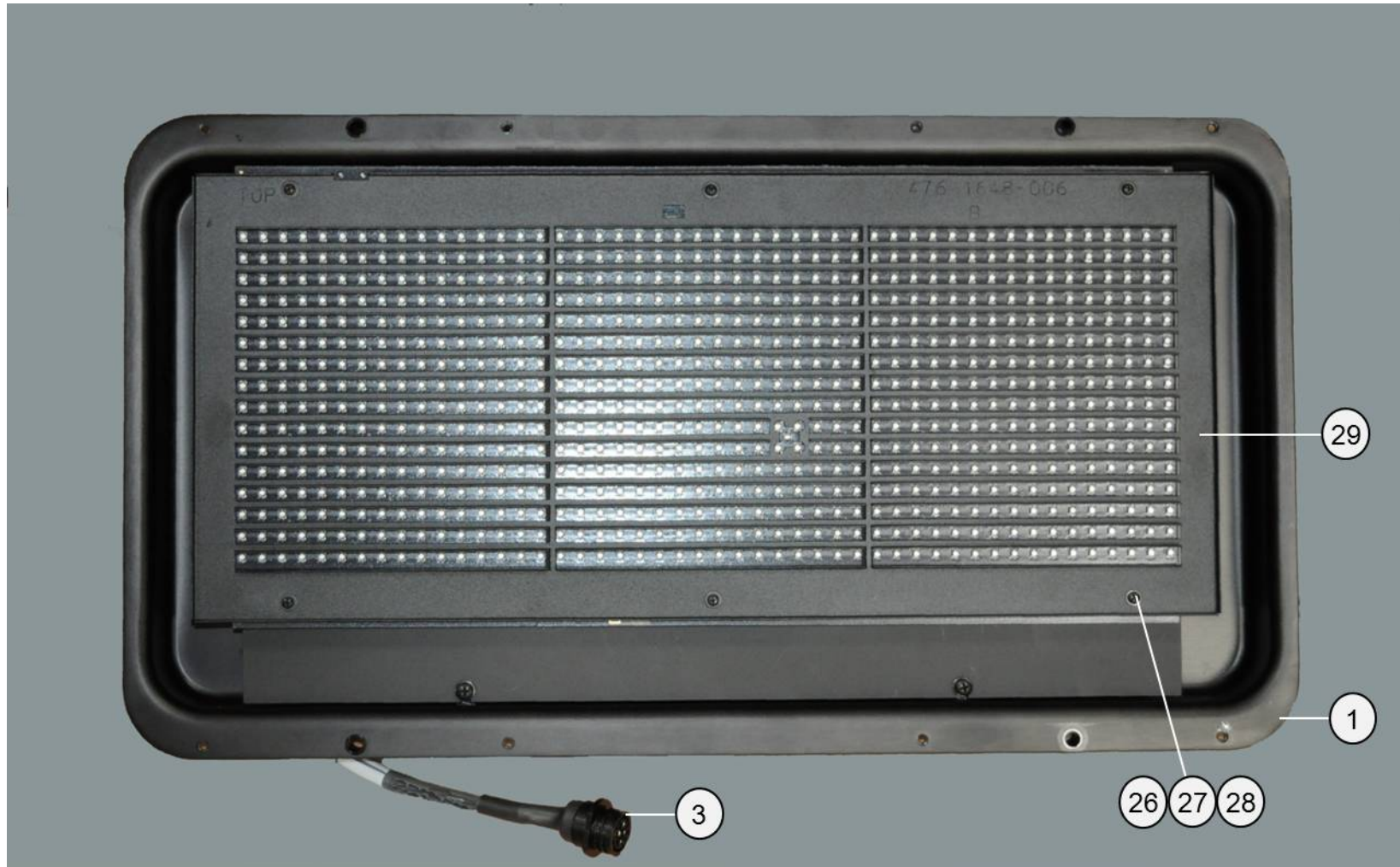
Figure 11-12. Hybrid Rear Sign, with Cover Removed
