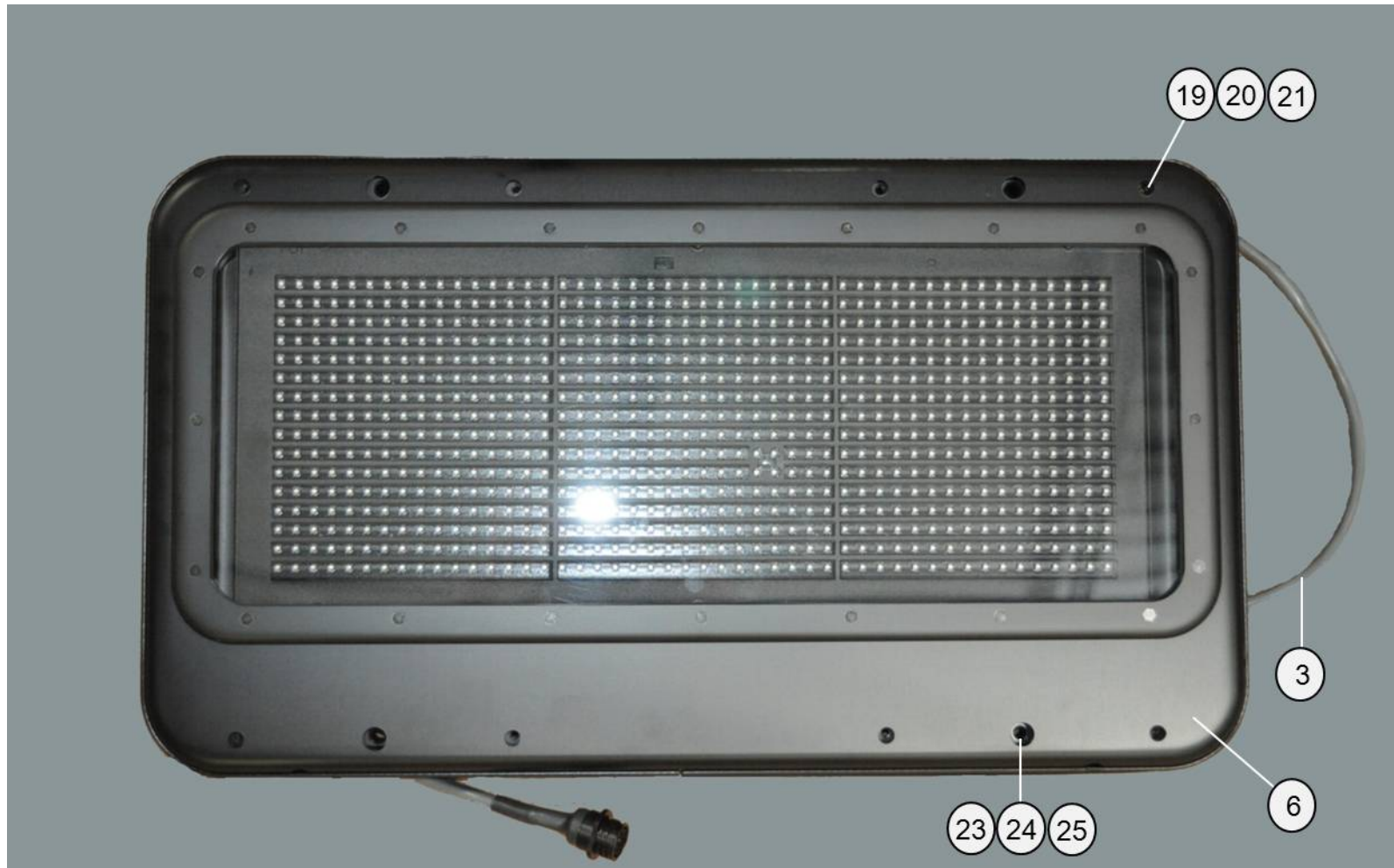
Figure 11-10. Hybrid Rear Sign, Front View
